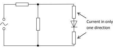
Hence only 2 resistors carry the current in 2 directions, and the resistors adjacent to the diode carry current in ONE direction only.
